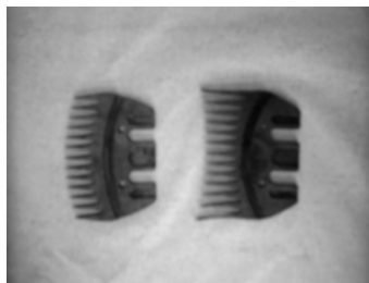
Figure 2: Shears: cutter and comb
