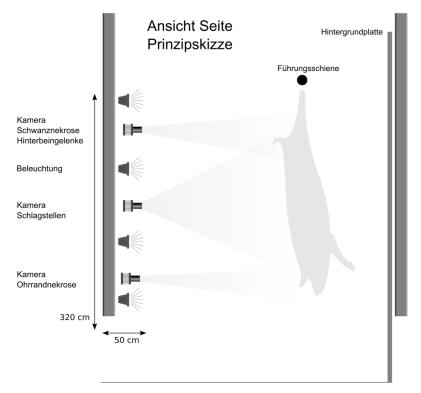
Fig. 1: Side view of the automated rating system (CLK GmbH)
