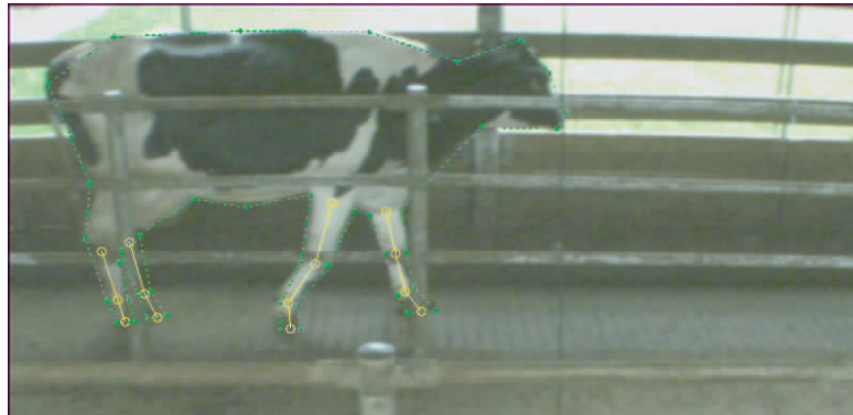
Fig. 4 Real time image-based model to calculate gait parameters for lameness detection
