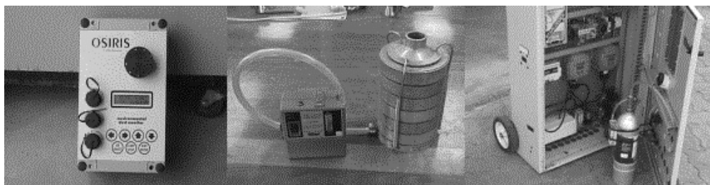
Figure 1. Measurement equipment used during the study included the (1) OSIRIS particle monitoring equipment, (2) Anderson bacteria sampler and the (3) Multi Gas Monitoring Machine, developed in-house.
